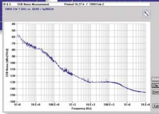
Typical SSB phase noise at f_c=1 GHz
